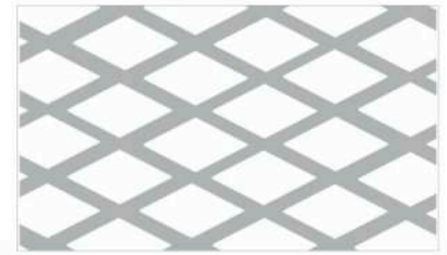
7 x 14mm - Alternada ec = 9,5mm EC= 21mm AA 49%
